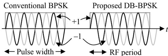
Fig. 2: Conventional and delay-based BPSK.
