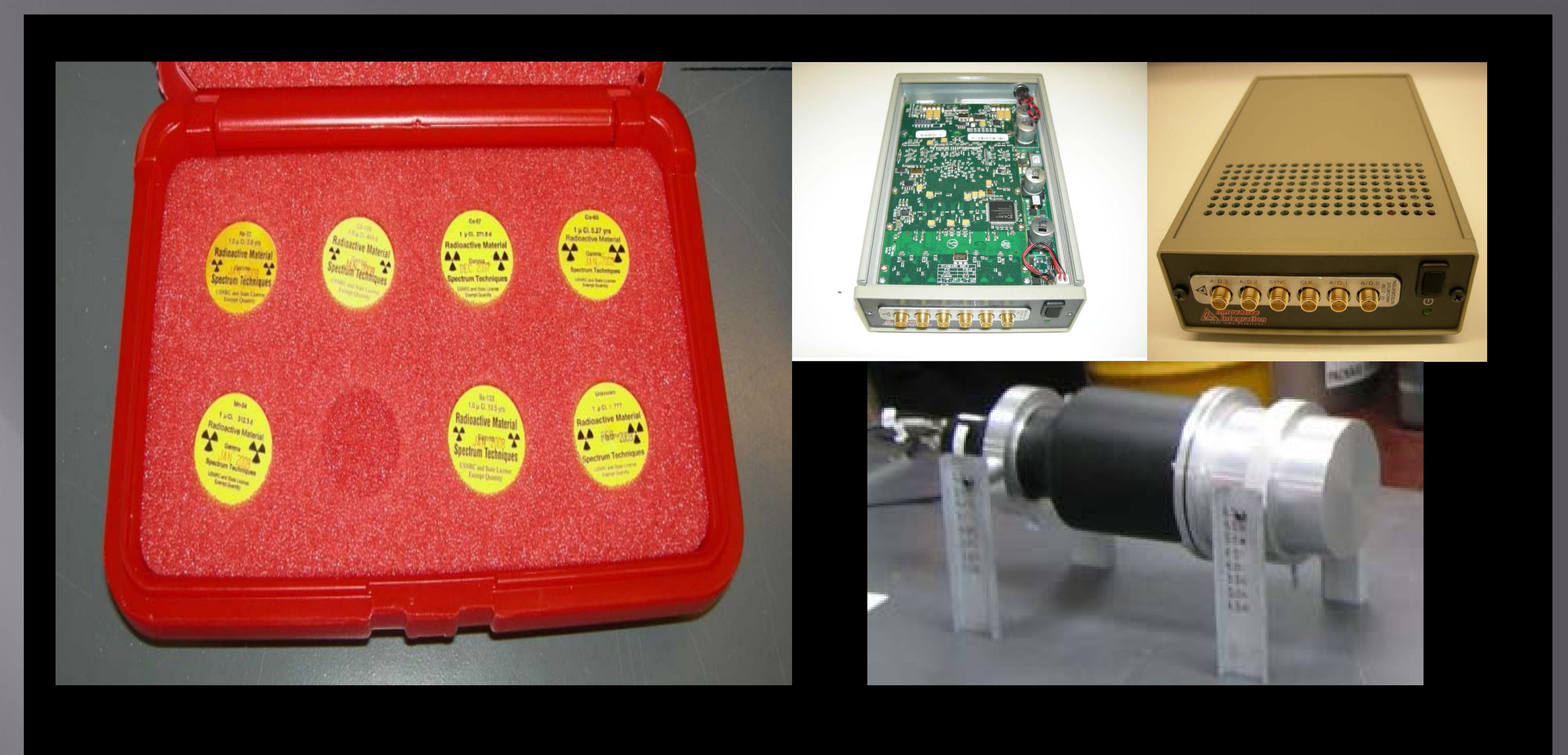
Figure 3. The University of Michigan developed a measurement system capable of acquiring the data on particles given off by radiation sources (left) with standard liquid scintillation detectors (bottom right) and a 250-MHz Innovative Integration (II) X5-210m digitizer (right).
