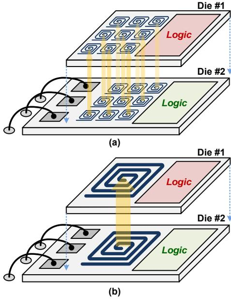
Fig. 4. Concept of parallel inductive power transfer (a) parallel power delivery using multiple maximum-power-density coils (b) single power delivery using one large coil
