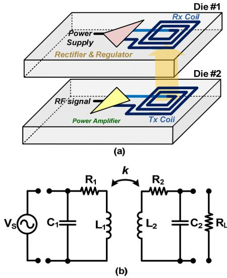
Fig. 2. (a) Concept of wireless inductive power link (b) Equivalent circuit
