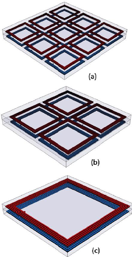
Fig. 9. Simulation setup for parallel inductive power link (a) 3x3 array of  $60\mu\text{m} \times 60\mu\text{m}$  coils (b) 2x2 array of  $90\mu\text{m} \times 90\mu\text{m}$  coils (c) single  $200\mu\text{m} \times 200\mu\text{m}$
