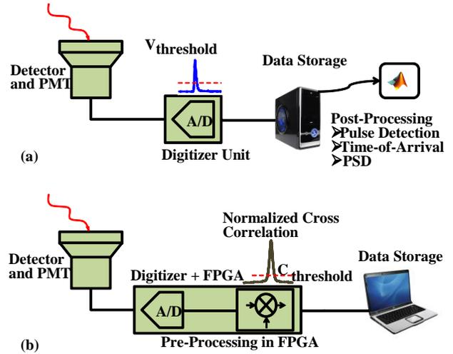
Figure 1: Block diagrams of (a) amplitude thresholding and (b) correlation based pulse detection technique
