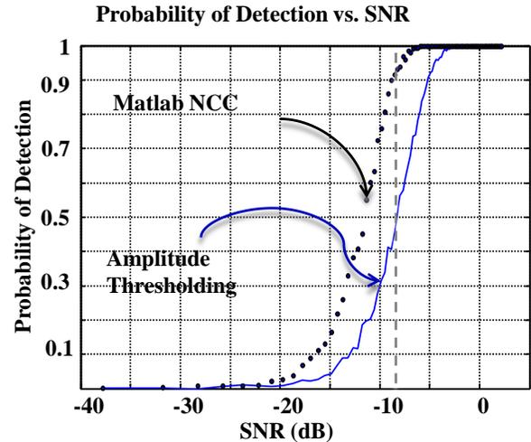
Figure 2: SNR vs. Probability of detection plot
